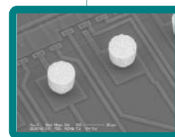
Medical application with 70µm-pitch flip chip
