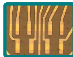
Medical application with 14µm lines and spaces
