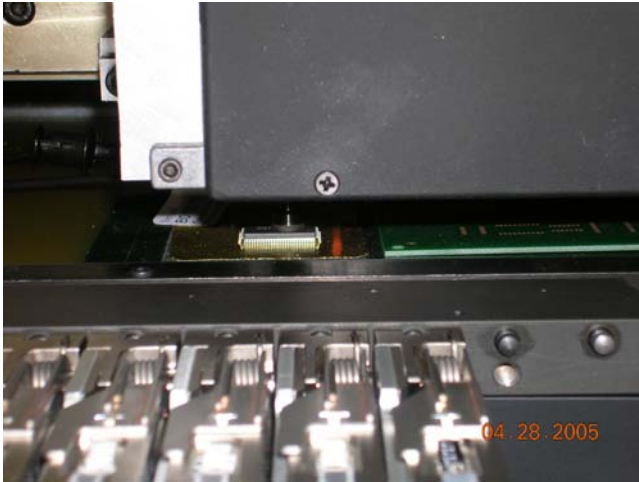
Photo 4 – placing charged device onto test board
