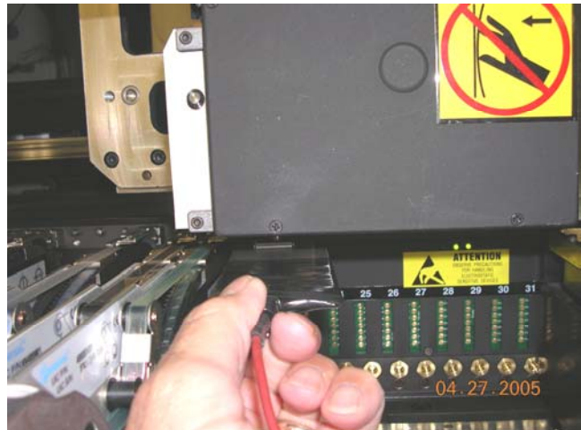
Photo 3 – applying a charge to a device in a handler
