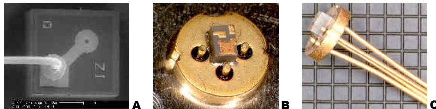
Figure 1: VCSEL assembly onto TO-header. (a) SEM of wirebonded VCSEL. (b) TO-header platform with laser submount. (c) TO-header with laser submount.
